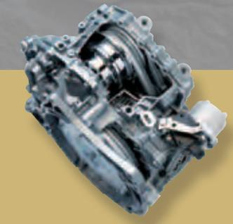
**CVT2.** CVT2 with AutoStick uses a 30-mm high-strength multilayer steel drive belt and two active V pulleys to vary vehicle speed. The result: a smooth, quiet ride that's very economical too.
